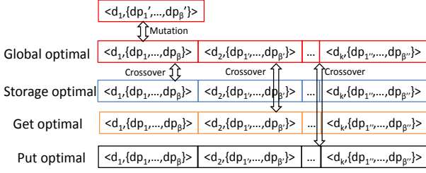
Fig. 4: GA-based data allocation adjustment.
