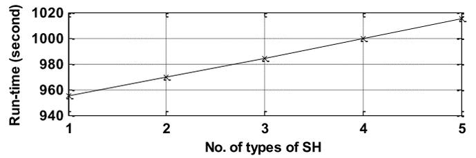
Fig. 22. Complexity analysis of the optimization algorithm presented for the GENCO based on the run-time (second) of the optimization algorithm with respect to the number of types of SH in the system.
