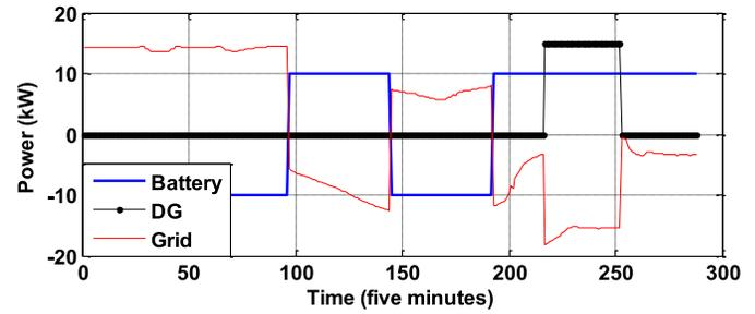
Fig. 18. Demand level and the optimally scheduled power of DG and battery at every 5-min step of the operation period (one day) for an SH with type 1 (after optimal EM).
