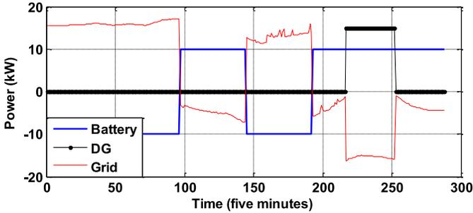
Fig. 14. Demand level and the optimally scheduled power of DG and battery at every 5-min step of the operation period (one day) for an SH with type 3 (before EM).
