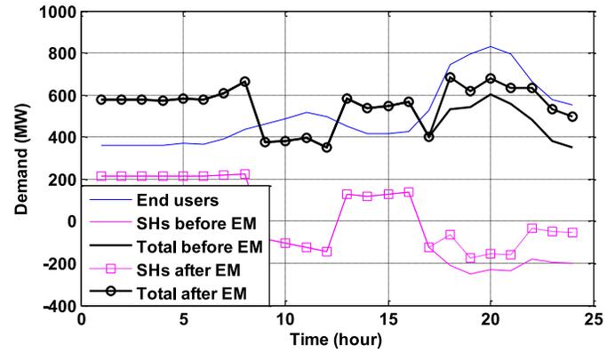
Fig. 17. Demand of passive end users, demand of active end users (SHs) before and after optimal energy management, and total demand of system before and after optimal energy management in MW at every hour of the operation period (one day).
