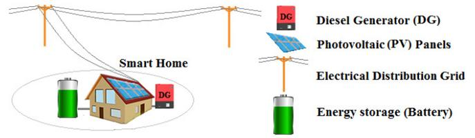
Fig. 6. Structure an SH that includes different energy resources.
