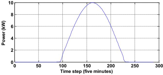
Fig. 8. Forecasted power pattern for the PV panels (type 1) in a purely sunny day at every 5-min step of the operation period (one day).
