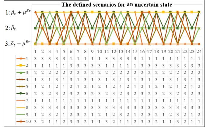
Fig. 4. Defined scenarios for the uncertain state of the problem (solar irradiance) at every time step (every 5 min) over the optimization time horizon (next 2 h).
