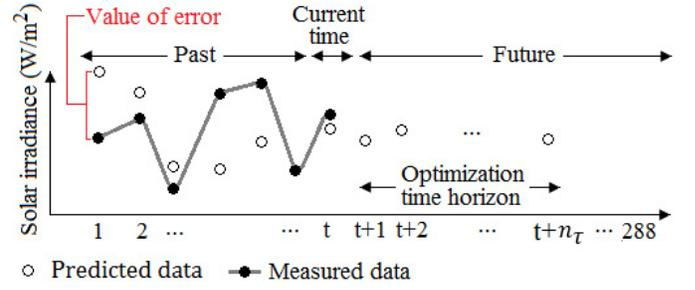
Fig. 3. Predicted data, measured data, and value of the prediction error.
