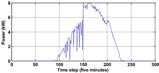
Fig. 9. Forecasted power pattern for the PV panels (type 2) in a cloudy day at every 5-min step of the operation period (one day).
