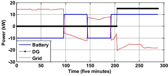
Fig. 13. Demand level and the optimally scheduled power of DG and battery at every 5-min step of the operation period (one day) for an SH with type 1 (before EM).
