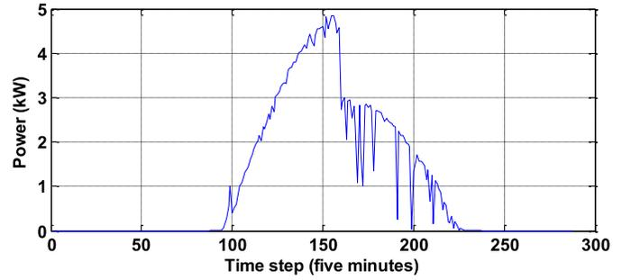
Fig. 10. Forecasted power pattern for the PV panels (type 3) in a cloudy day at every 5-min step of the operation period (one day).
