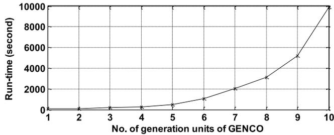
Fig. 21. Complexity analysis of the optimization algorithm presented for the GENCO based on the run-time (second) of the optimization algorithm with respect to the number of generation units of the GENCO.
