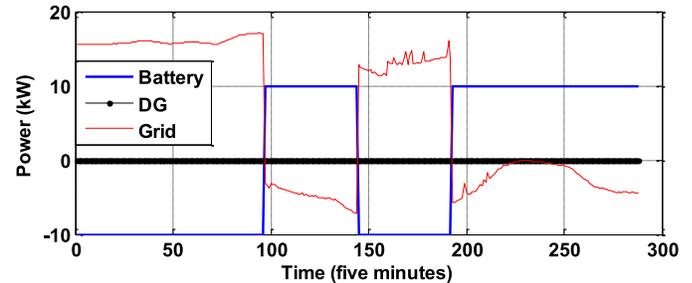
Fig. 19. Demand level and the optimally scheduled power of DG and battery at every 5-min step of the operation period (one day) for an SH with type 3 (after optimal EM).
