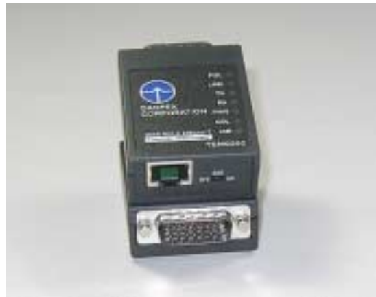
Figure 3. Two AUI/RJ-45 transceivers – the top one shows the RJ-45 end, the bottom one shows the AUI end.
