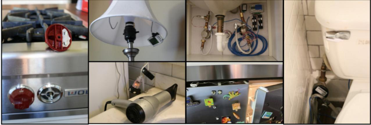
**Figure 2. Sensor Deployment:** All major electrical and water fixtures in the test home were instrumented. The stove knobs and fridge doors were fitted with rare earth magnets, and detected by reed switch sensor. Light fixtures were monitored with optical fiber based directional light sensor. Appliances such as hair dryer, were detected using power meters. Sinks and toilet flush tanks were instrumented with in-line water flow sensors
