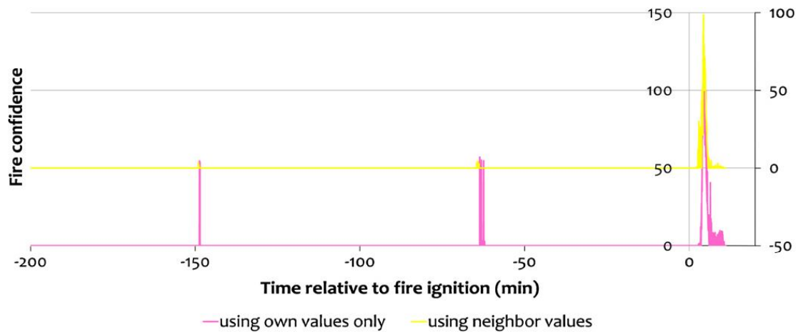
Fig. 9. Simulating a burning chair: including neighbor readings in the decision. The results when only own values are used are plotted on the first y-axis. Including the neighbor values is plotted on the second y-axis.
