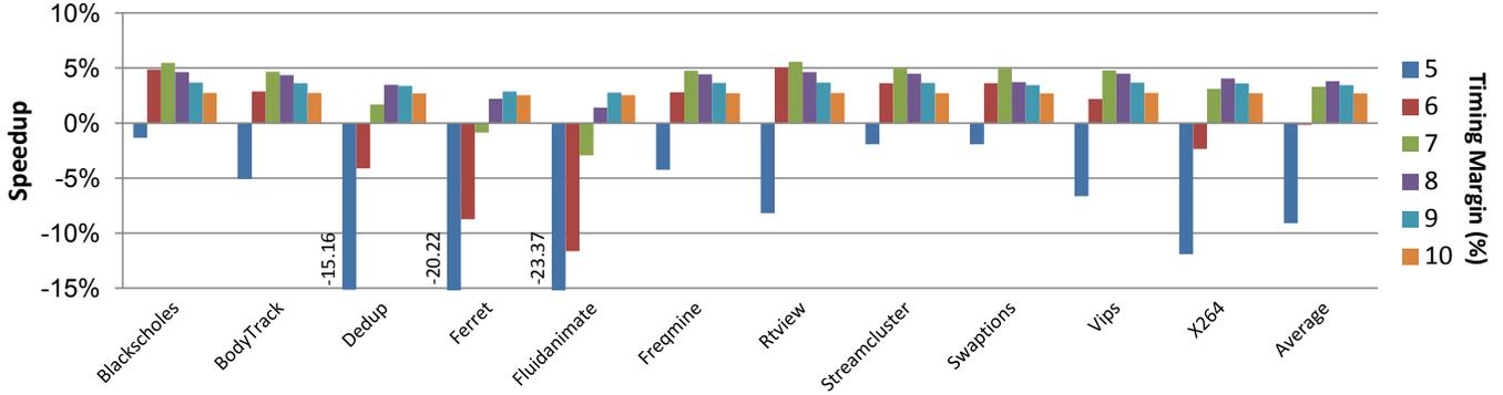
**Figure 7: Speed up of recovery-based techniques with different timing margin settings. We evaluate our 16nm, 16core processor with 24MCs here. The baseline case enforces a 13% timing margin and thus guarantees timing is error-free.**
