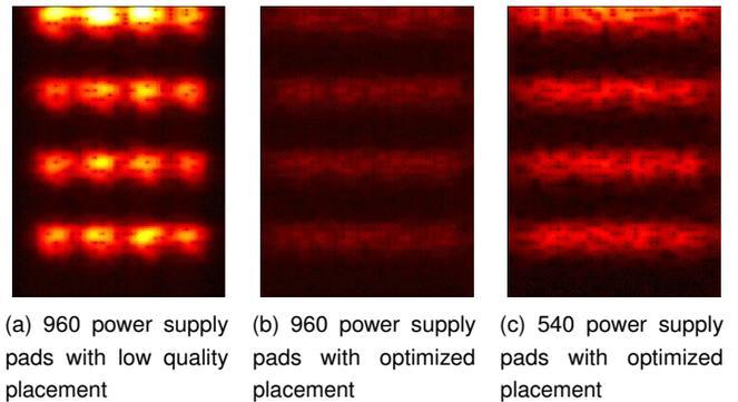
**Figure 2: Voltage-emergency maps for different pad configurations for a 16nm, 16-core chip. A total of 1914 C4 locations are available. All three graphs have the same color scale; areas with warmer colors indicate more voltage violations.**
