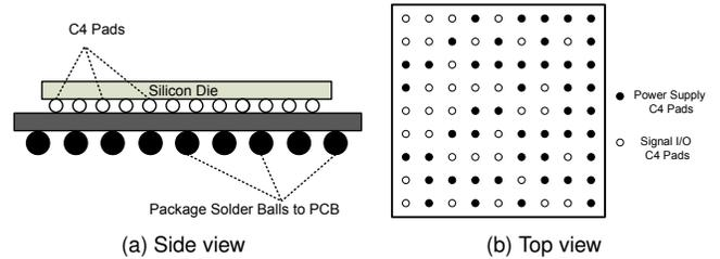
**Figure 1: (a) Side view of a chip showing its connection to the package through C4 pads. (b) Top view of a C4 array showing an example allocation of power pads and I/O pads (real processors have many more C4 pads than illustrated here).**
