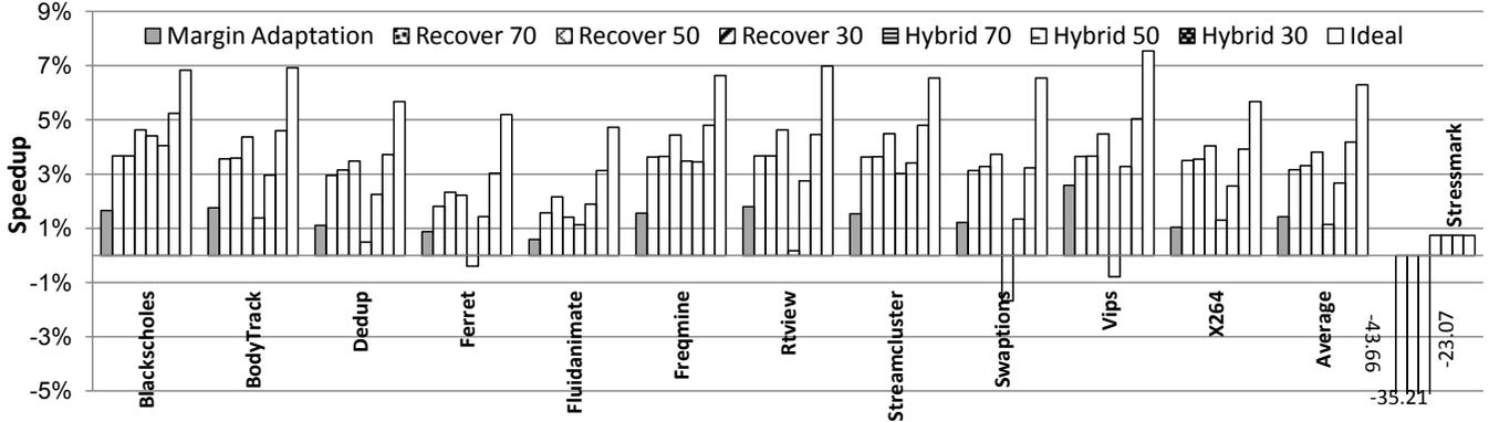
**Figure 8: Performance comparison between different noise mitigation techniques. Numbers after recover/hybrid in legend represent the cost (in cycles) of each recover, from error. The baseline case enforces a 13% constant timing margin.**
