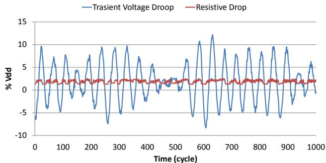
Figure 5: Comparison of transient voltage noise and static IR drop over a 1K cycle window in the benchmark ferret. Periodic oscillation implies that  $LC$  resonance is the major cause. We build our noise-inducing stressmark based on this segment.
