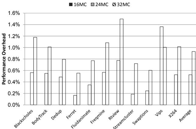
**Figure 9: Performance penalty of mitigating extra voltage noise caused by reduced power/ground pads. We use the hybrid technique with a conservative assumption of 50-cycle rollback-and-replay penalty per error. Each benchmark uses its own performance with 8MC case as baseline.**
