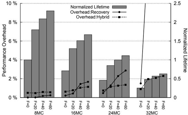
**Figure 10: PDN pad failure’s effect on noise mitigation performance overhead and expected EM lifetime.**  $F$  indicates the number of failed pads. The baseline is an 8 MC chip with no failed pads. For *Recovery*, the performance overhead with 32 MC goes off-chart to 15% if 20 pads fail (25% if 60 pads fail).
