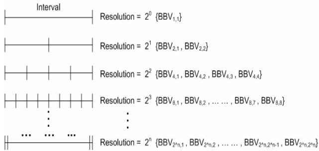
Figure 6. Basic Block Vectors (BBVs) that represent the same program execution interval at different resolutions (The coarser scale BBVs are the approximations of the finest scale BBVs generated by the wavelet-based multiresolution analysis)
