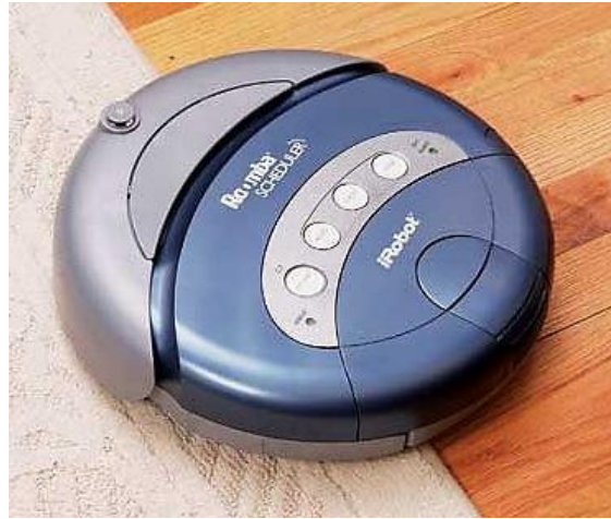
“Roomba” autonomous vacuum, by iRobot, 2002
