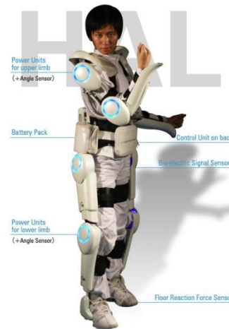
Cyberdyne’s HAL-5 exoskeleton, 2006 51 lbs, runs 5 hrs, cost: $60K or $600/mo 5x strength amplification
