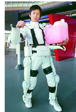
Cyberdyne’s HAL-5 exoskeleton, 2006 51 lbs, runs 5 hrs, cost: $60K or $600/mo 5x strength amplification
