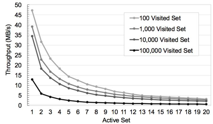
Fig. 3. Sensitivity of automata simulation performance to changes in the active set (number of states considered per cycle) and the visited set (number of states consistently visited). Performance is much more sensitive to increases in active set. The visited set impacts performance when its size grows larger than the size of an available level of cache.
