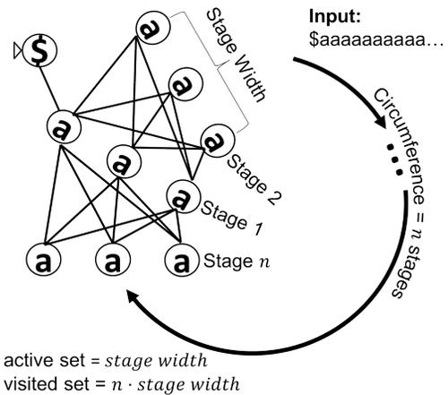
Fig. 2. Parameterizable synthetic automata design. Each ring is guaranteed to have a constant active set and visited set, and is driven by an easy-to-generate input string. This instance has width 3, thus active set 3. Each stage is fully connected with its succeeding stage to form a continuous ring. The circumference,  $n$ , is derived using the equation  $n = \lceil \frac{\text{visited}}{\text{width}} \rceil$ .
