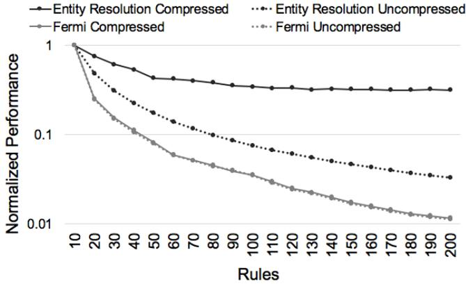
Fig. 1. Sensitivity of VASim performance in response to additional automata rules. Performance of automata with many common prefixes and high activity compressability (ER) are less sensitive to additional rules. This indicates average automata activity after common optimizations, rather than total rule-count, is a better predictor of performance.
