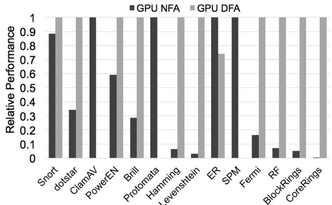
Fig. 6. Relative performance of NFA and DFA engines over all benchmarks in ANMLZoo. DFAs for ClamAV, Protomata, and SPM were too expensive to construct due to space or time costs.
