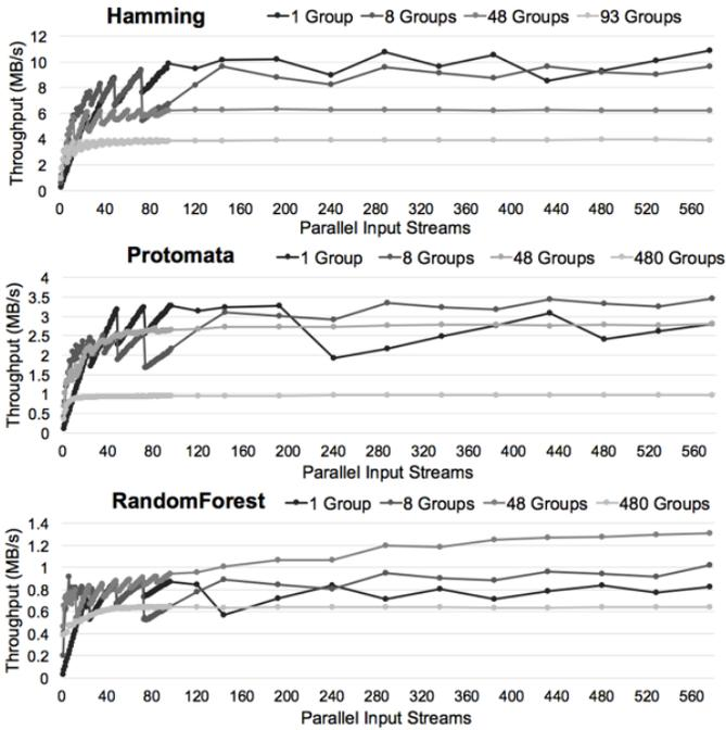
Fig. 5. Protomata, Hamming, and Random Forest all benefit from a massive amount of stream level parallelism, however appropriate care must be taken to tune automata groups to match GPU core resources.
