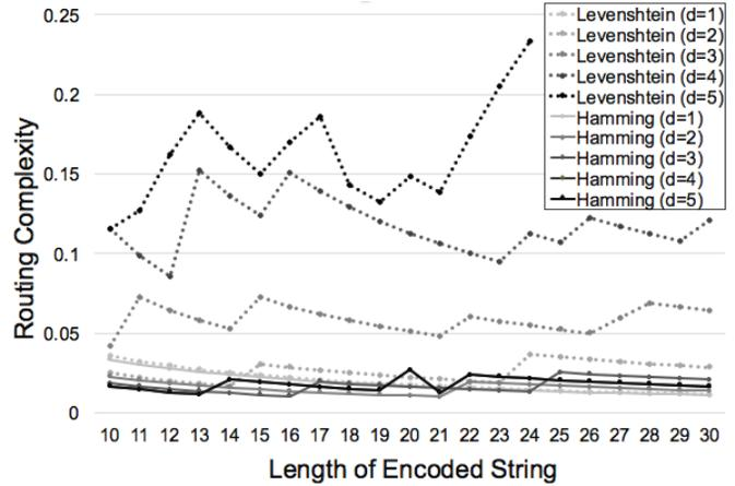
Fig. 7. Hamming automata have a constant fan-in/fan-out per STE and therefore have relatively low routing complexity that is not impacted by the dimension of the mesh. The node degree of Levenshtein automata grows linearly in the size of the encoded edit distance threshold, therefore routing complexity is very sensitive to this dimension.
