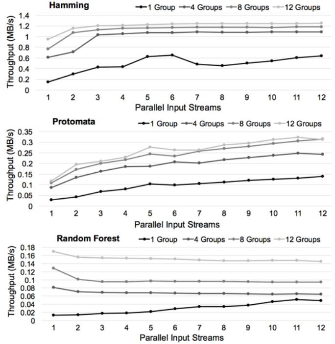
Fig. 4. Hamming automata benefit most from automata-level parallelism. Protomata benefits from parallelism in both dimensions. Random Forest only benefits from automata-level parallelism.
