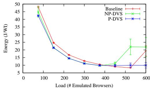
Figure 3.7: Comparison of total system energy per web interaction [36, Fig. 7].
