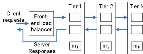
Figure 3.1: General model of clustered multi-tier system [36, Fig. 1].
