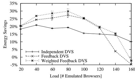
Figure 2.9: Total DVS energy savings (TPC-W workload) [35, Fig. 13].
