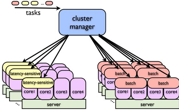
**Figure 3: Task placement in a cluster. The cluster manager does not co-locate latency-sensitive applications with others to protect their QoS from performance interference, causing low machine utilization.**
