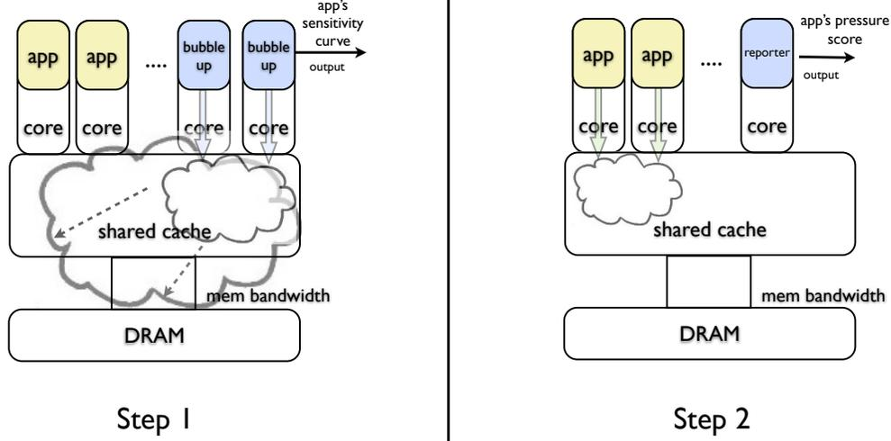
**Figure 4: Bubble-Up Methodology.** In Step 1, we characterize the *sensitivity* of the host application task to pressure in the memory subsystem using a *bubble*. In Step 2, we characterize the *contentiousness* of the host application in terms of the amount of pressure it causes on a *reporter*.
