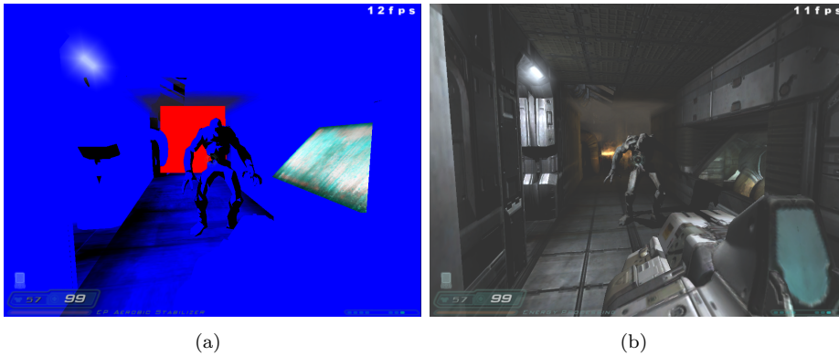
Figure 3. Screen captures from the doom3 benchmark. On the left, the color of each pixel is modulated to indicate which fragment program generated it. The right image is the unmodified rendering from the game. Notice that the majority of pixels are generated by programmable fragment shaders.
