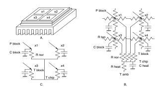
Figure 3. IC die with 4 functional blocks.
