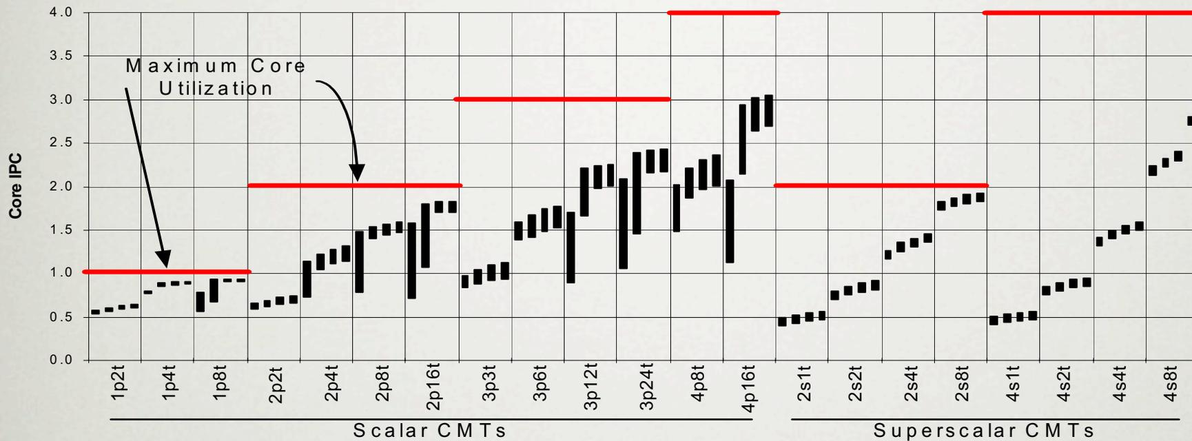
Scalar CMT cores outperform Superscalar CMT cores due to the additional scalar cores that fit the area budget
