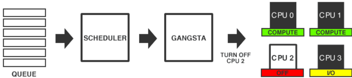
Figure 1: A graphical overview of our system. Processes exist in a process queue. A black-box scheduler schedules these processes as it normally would. GANGSTA receives the scheduled jobs and decides whether to turn cores on or off depending on the execution state of each core and the processes handed to it by the black-box scheduler.
