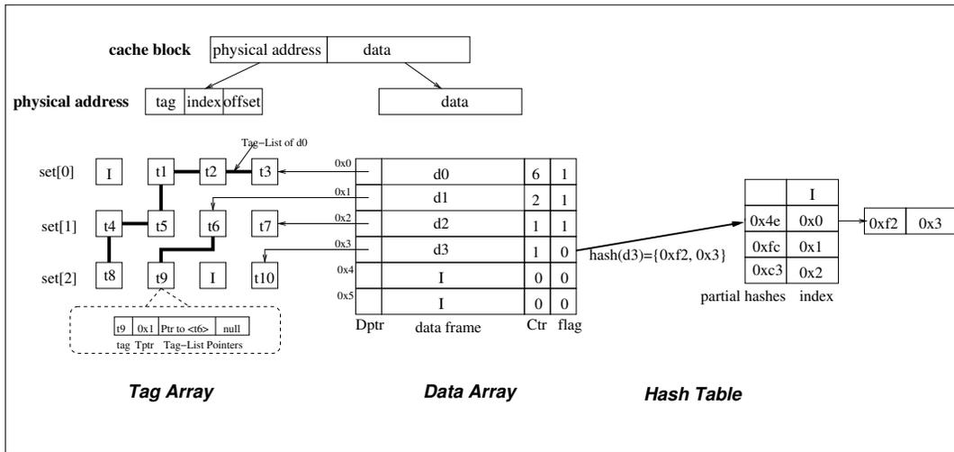
Figure 3: Structure of a deduplicated LLC. Blocks t1, t2, t3, t4, t5 and t8 are duplicated blocks, sharing identical data d0; t6 and t9 share data d1; t7 is a distinct block with data d2; and, t10 is inserted as a distinct block and has not been analyzed for deduplication yet.
