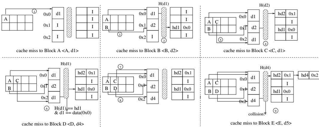
Figure 4: An example of hash-based post-process last-level cache deduplication.
