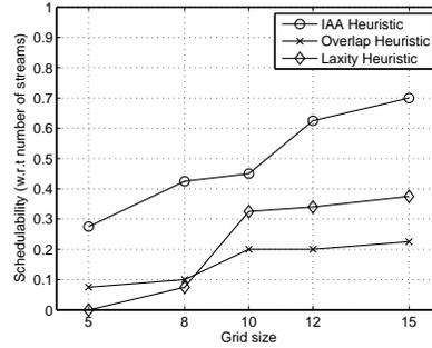
(a) Deadline tightness of 3, 40 streams: The laxity heuristic lags behind the overlap heuristic. But it shows an upward trend as grid size increases.
