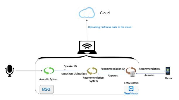
FIGURE 1. The Overview of the PCR system with its four major components: the Acoustic Pipeline, the Recommendation System, and EMA system, and M2G.
