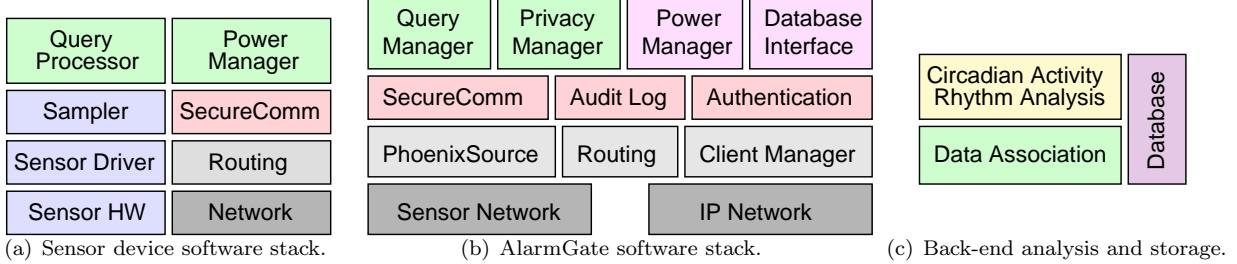
Figure 1.3: AlarmNet component software.
