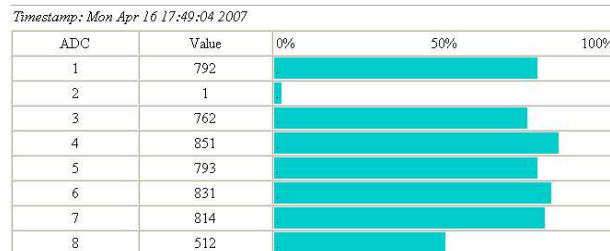
Figure 2. LUSTER web server generated page reporting ADC levels for a pre-selected remote sensor node.
