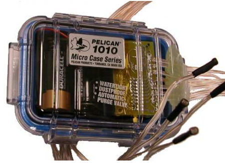
Figure 9. Packaged “Medusa” sensor module.
