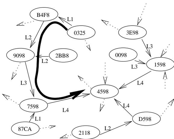
**Figure 3: A portion of the global mesh, rooted at node 4598. Paths from any node to the root of any tree can be traversed by resolving the root’s ID one digit at a time; the bold arrow shows a route from node 0325 to node 4598. Data location uses this structure. Note that most object searches do not travel all the way to the root (see text).**
