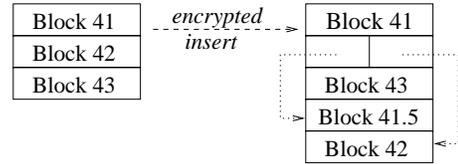
**Figure 4: Block insertion on ciphertext.** The client wishes to insert block 41.5, so she appends it and block 42 to the object, then replaces the old block 42 with a block pointing to the two appended blocks. The server learns nothing about the contents of any of the blocks.
