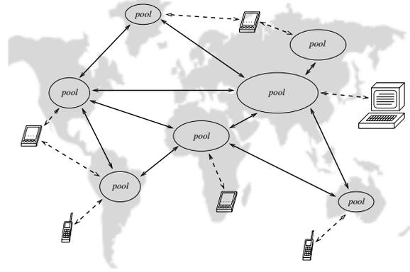
**Figure 1: The OceanStore system.** The core of the system is composed of a multitude of highly connected “pools”, among which data is allowed to “flow” freely. Clients connect to one or more pools, perhaps intermittently.
