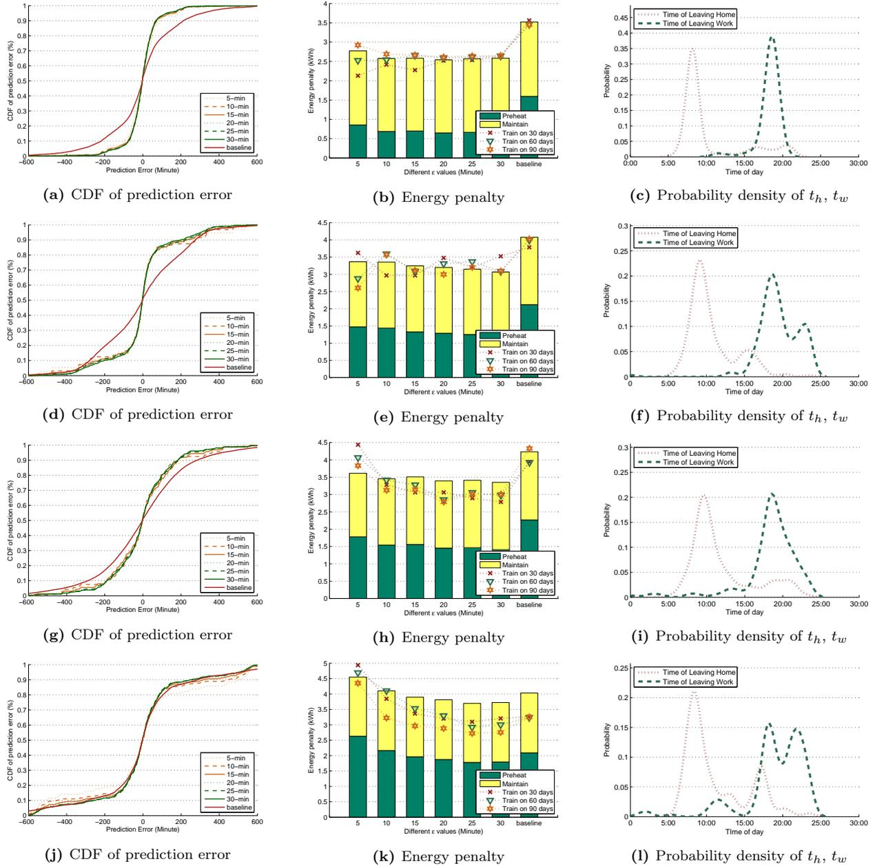
**Figure 1:** Each row contains the results for one user: the first column is the CDF of prediction error distribution for arrival times; the second column is the energy penalty, the optimal case of each user has energy savings ranging from 8.3% to 27.9% than baseline; the last column is the probability distribution of each user’s leaving home times and leaving work times.
