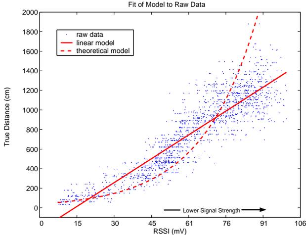
Figure 4: **RSSI Models** The linear model does not capture the 'dip' near the middle of the curve. However, the theoretical model creates huge errors, especially for the RSSI measurements near 90mV, which are taken near 10m, but are estimated to be 20 or 30m.
