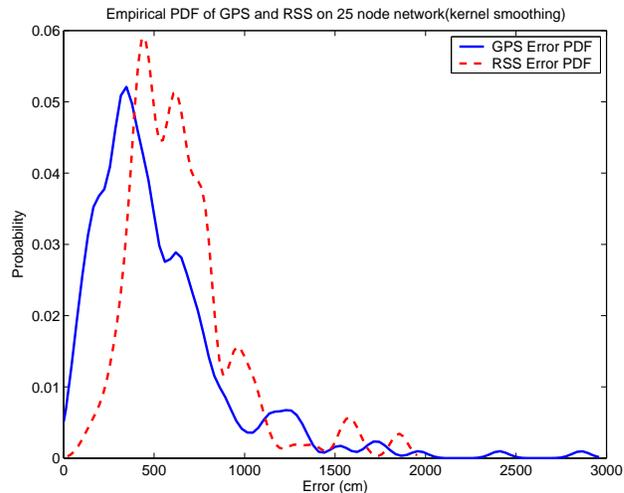
Figure 7: **Error PDFs** GPS has lower mean error, but has outliers of up to 30m. RSS has a slightly higher average error, but smaller magnitude outliers.
