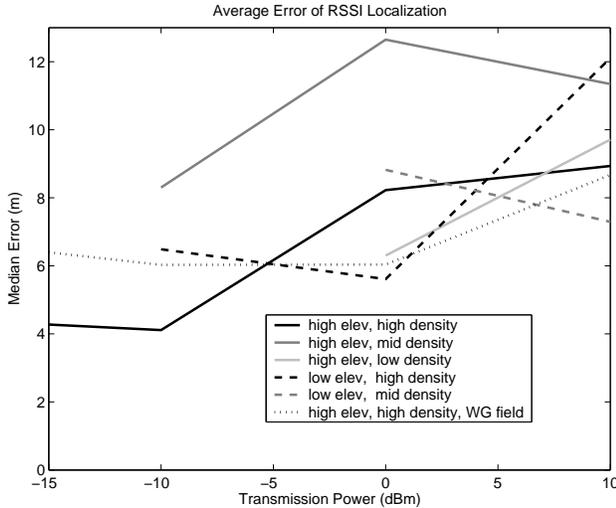
Figure 6: **Median Errors** This plot depicts the median error for each of 35 deployment scenarios. At points not plotted, the network did not successfully localize.
