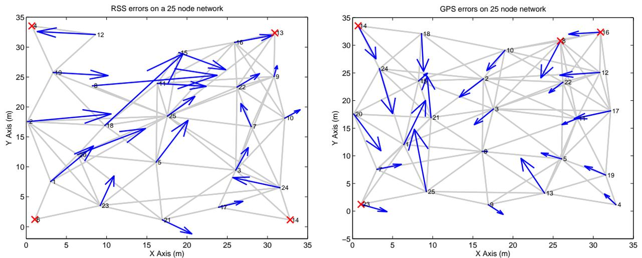
Figure 9: **25 Node network** Edges in the left graph indicate radio connectivity, in the right graph they indicate distances of 10m or less. In the 25 node network, RSS localization (left) performs well except in the face of connectivity holes (top left corner). GPS has problems with surrounding buildings and trees, which do not effect RSS.
