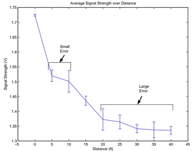
Figure 1: **Error Increase over Distance** depends on both noise and attenuation rate. As the signal strength flattens out, differences in signal strength become small relative to noise levels.
