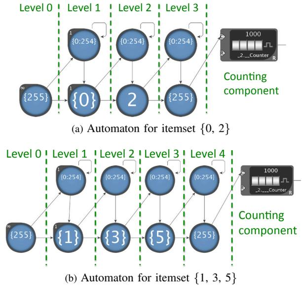
Figure 2: Initial design of automata for ARM itemset matching and support-counting. Blue circles and black boxes are STEs and counters, respectively. The numbers on an STE represent the symbol set that STE can match. “0:254” means any item ID in the range of 0-254. Symbol “255” is reserved as the transaction separator.
