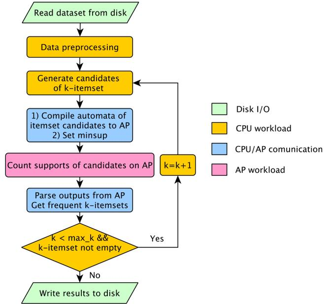
Figure 1: The workflow of AP-accelerated ARM
