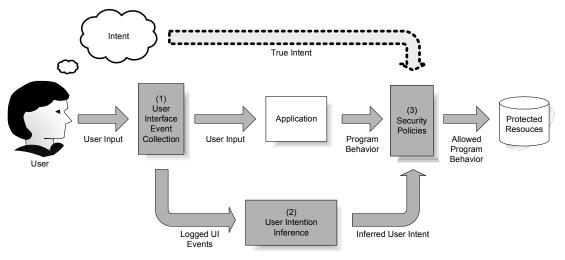
Figure 1. User-Intent-Based Access Control
