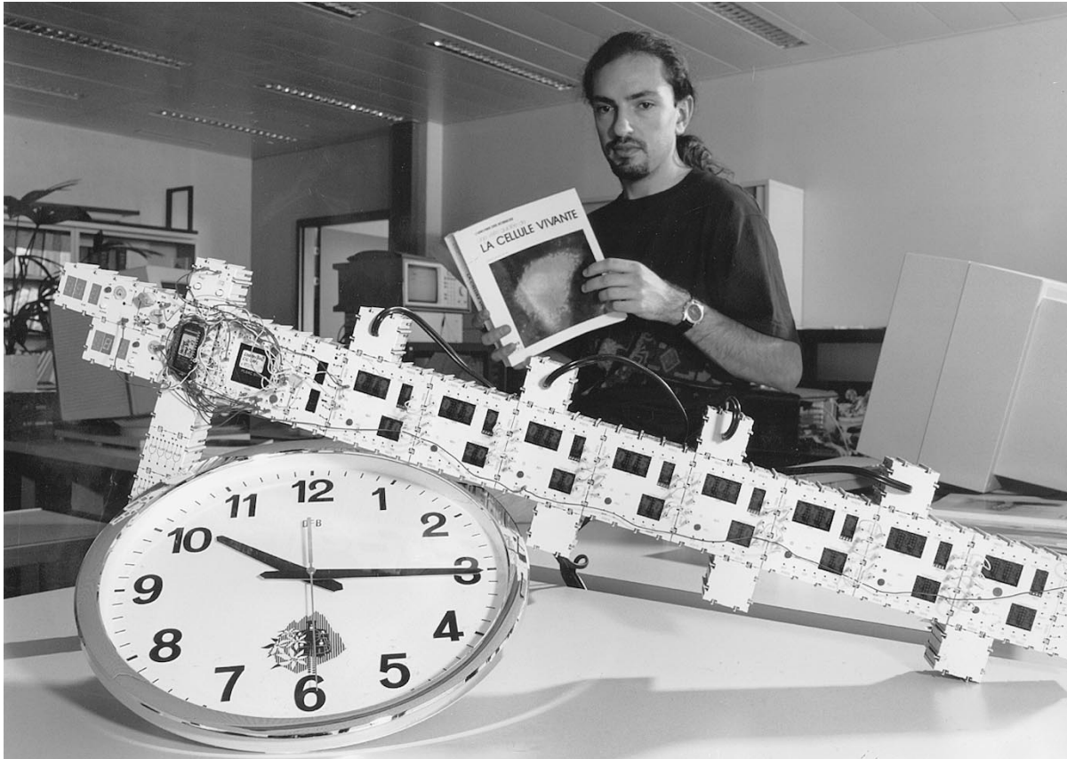
Fig. 14. BioWatch, a full digital watch. (a) Multicellular organization ( X=1 : tens of hours; X=2 : units of hours). (b) Experiment with eight MICTREE cells and two spare cells.
