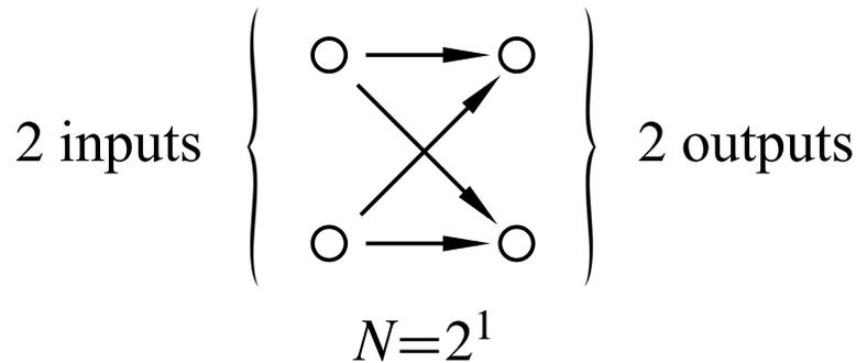
**Figure 10.1**  $F_1$ , the Butterfly Net switches with  $N = 2^1$ .
