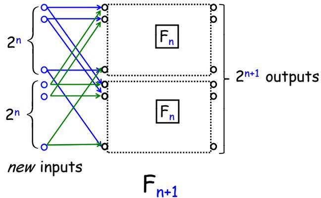
**Figure 10.2**  $F_{n+1}$ , the Butterfly Net switches with  $2^{n+1}$  inputs and outputs.
