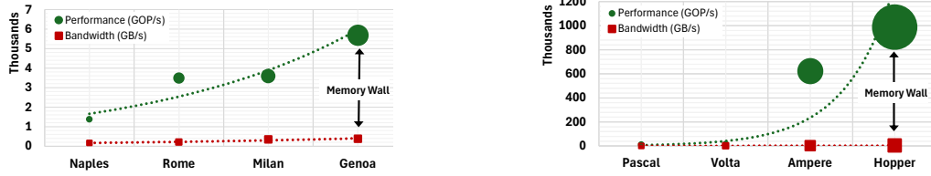
(a) Performance and bandwidth scaling for AMD EPYC CPUs. While performance increases by \sim 4\times from Naples to Genoa, memory bandwidth improves by \sim 2\times .
