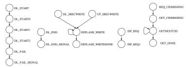
Figure 17. XNP state machines. The names of the states are from the code. The IDLE and ACK states are not shown.
