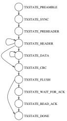
Figure 19. Transmission state machine from the SOS CC1000 driver.
