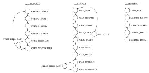
Figure 18. Three state machines from TinyDB.
