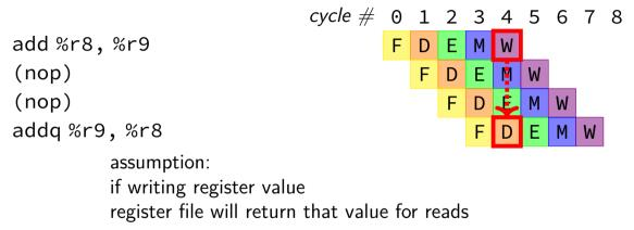
not actually way register file worked in single-cycle CPU (e.g. can read old %r9 while writing new %r9)
