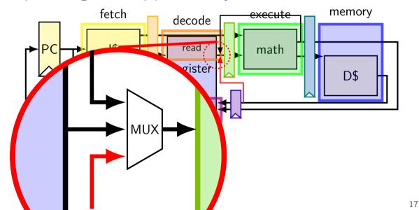
exercise: forwarding paths cycle # 0 1 2 3 4 5 6 7 8 addg %r8, %r9 FDEMW FDEMW subg %r8, %r10 xorq %r8, %r9 FDEMW andg %r9, %r8 FDEMW in subg, %r8 is \_\_\_\_\_ addg. in xorq, %r9 is \_\_\_\_\_ addq. in andg, %r9 is \_\_\_\_\_ addg.
