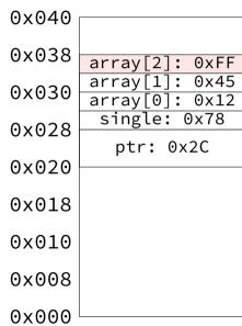
int  $array[3] = \{0x12, 0x45, 0x67\};$ int single = 0x78; int \*ptr; ptr = &arrav[0];ptr[2] = 0xFF: \*(ptr + 2) = 0xFF;int \*temp1; temp1 = ptr + 2;  $\star temp1 = 0xFF$ : int \*temp2; temp2 = &ptr[2];  $\star temp2 = 0xFF:$
