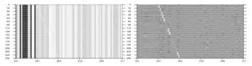
Fig. 5. Prime+Probe attack using 30,000 encryption calls on a 2GHz Athlon 64, attacking Linux 2.6.11 dm-crypt. The horizontal axis is the evicted cache set (i.e.,  $\langle y \rangle$  plus an offset due to the table's location) and the vertical axis is  $p_0$ . Left: raw timings (lighter is slower). Right: after subtraction of the average timing of the cache set. The bright diagonal reveals the high nibble of  $p_0 = 0x00$ .
