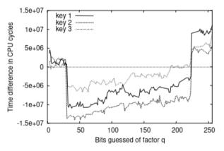
(a) The zero-one gap  $T_g - T_{g_{hi}}$  indicates that we can distinguish between bits that are 0 and 1 of the RSA factor q for 3 different randomly-generated keys. For clarity, bits of q that are 1 are omitted, as the x-axis can be used for reference for this case.
