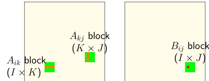
$B_{ij}$  calculation uses strips from  $A$
