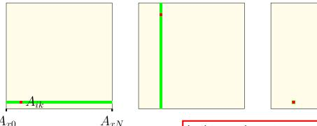
looking only at innermost loop: row of A (elements used once) column of B (elements used once) single element of C (used many times)
