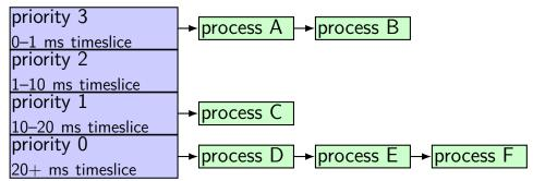
goal: place processes at priority level based on CPU burst time just a few priority levels — can't guess CPU burst precisely anyways
