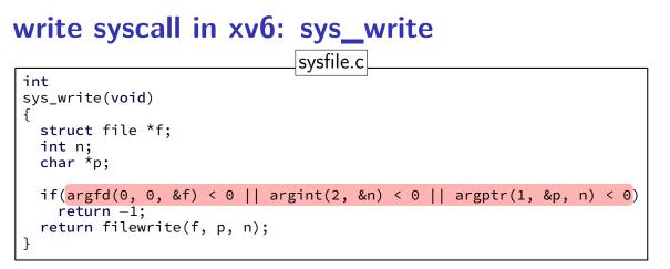
utility functions that read arguments from user's stack returns -1 on error (e.g. stack pointer invalid) (more on this later) (note: 32-bit x86 calling convention puts all args on stack)
