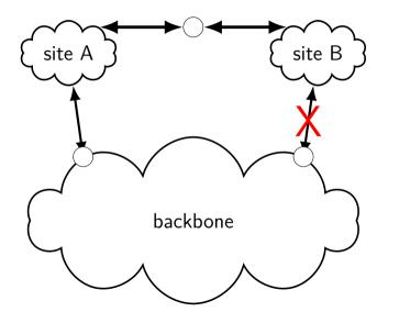
if B's link to backbone fails, B should use building A's
