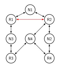
can have direct router-router link
