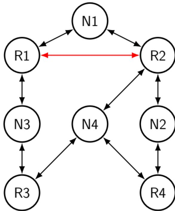
can have direct router-router link
