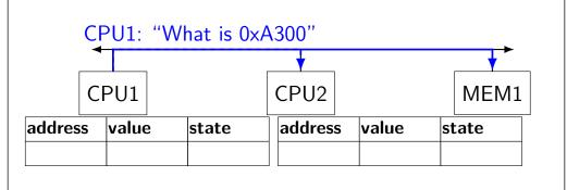
CPU1: read 0xA300 CPU1: write 0xA300 CPU1: read 0xA300 CPU2: read 0xA300 CPU2: write 0xA300
