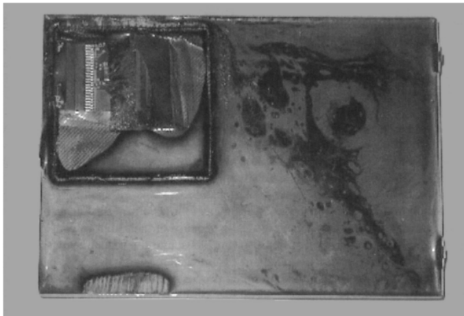
Figure 14.2 The 4758 partially opened, showing (from top left downward) the circuitry, aluminium electromagnetic shielding, tamper-sensing mesh and potting material (courtesy of Frank Stajano).
