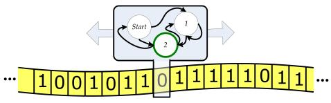
Figure 6.6. Turing Machine model.
