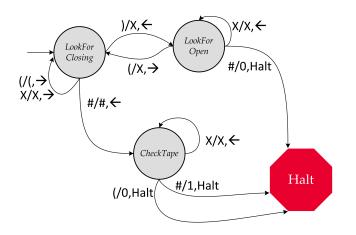
Figure 6.8. Checking parentheses Turing Machine.
