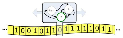
Figure 6.7. Turing Machine model.
