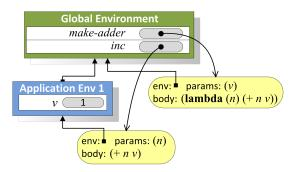
Figure 10.3. Environment after evaluating (define inc (make-adder 1)).
