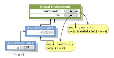
Figure 10.4. Environment for evaluating the body of (inc 149).
