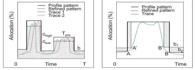
(a) Pattern refinement by lowering (b) Pattern refinement by varying the the cap. base provision.
