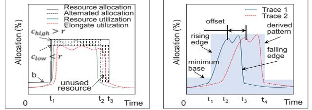
(a) Elastic resource provisioning. (b) Rising, falling edges and pulse deviation.
