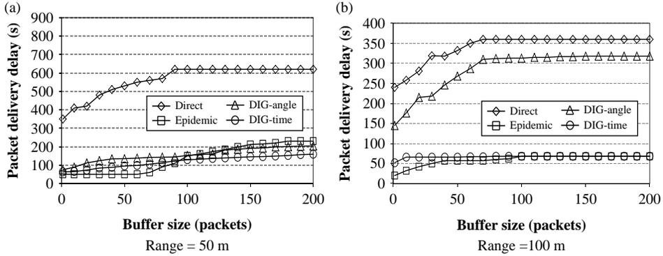
Figure 6. Packet delivery delay versus buffer size in HMM.
