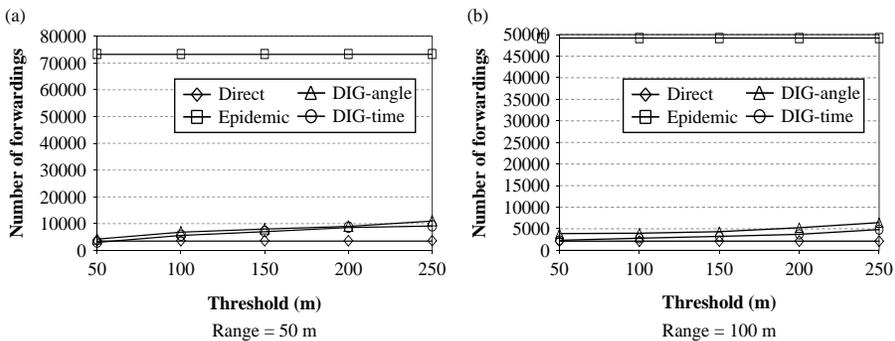
Figure 18. The number of forwardings versus threshold in HMM.
