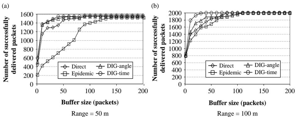
Figure 8. The number of successfully delivered packets versus buffer size in HMM.
