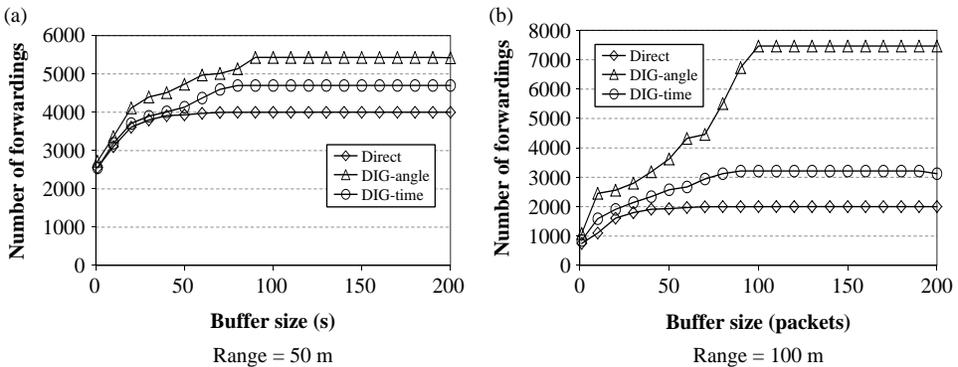
Figure 12. The number of forwardings versus buffer size in HMM.
