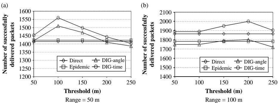
Figure 16. The number of successfully delivered packets versus threshold in HMM.
