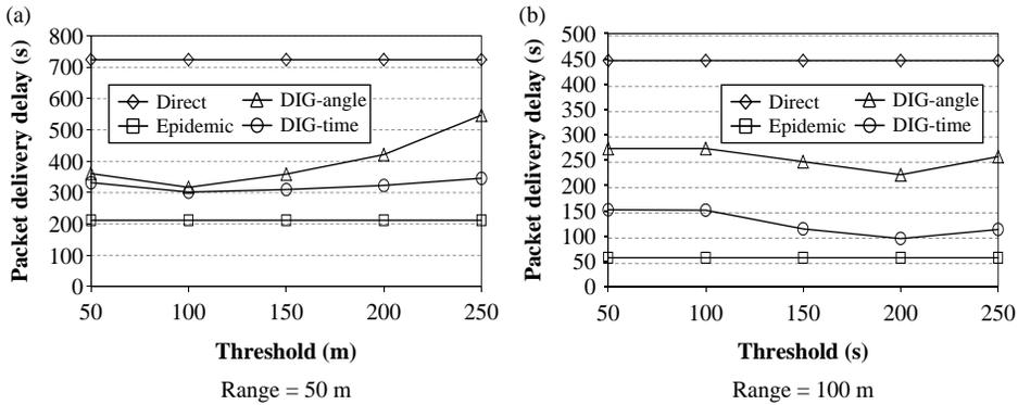
Figure 13. Packet delivery delay versus threshold in UMM.
