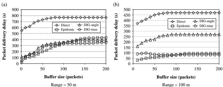
Figure 5. Packet delivery delay versus buffer size in UMM.
