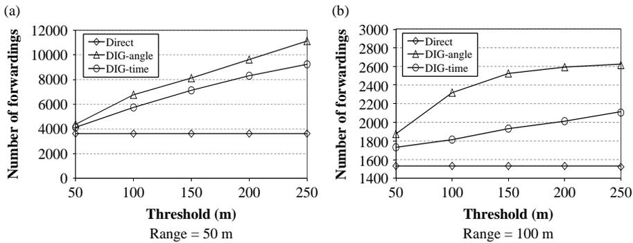
Figure 19. The number of forwardings versus threshold in UMM.
