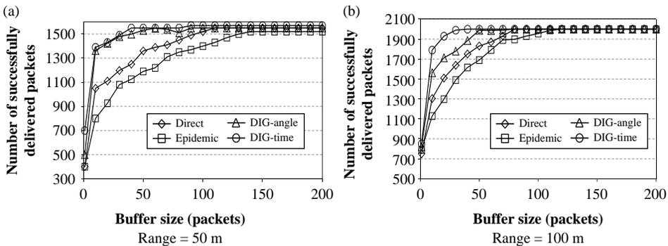
Figure 7. The number of successfully delivered packets versus buffer size in UMM.
