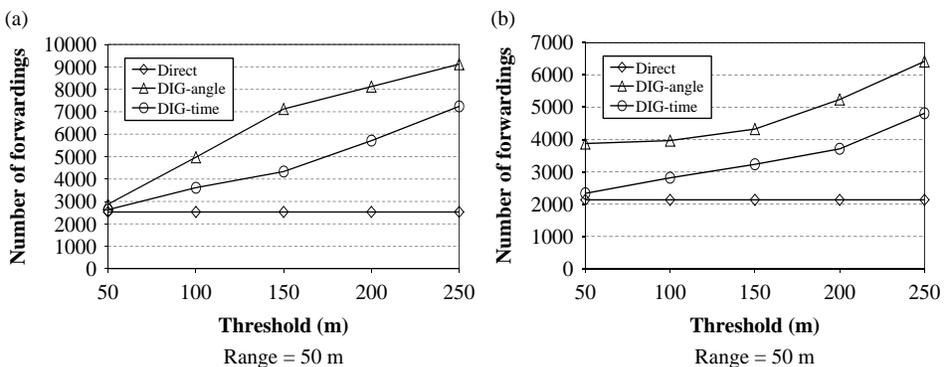
Figure 20. The number of forwardings versus threshold in HMM.
