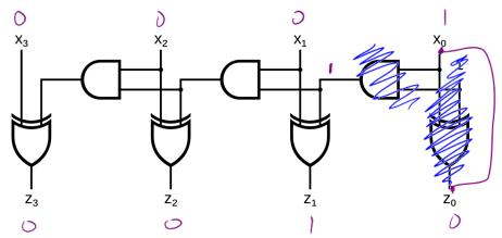
How can we change this circuit to instead increment by 2, i.e., x += 2? Draw the new circuit below. Note: you should not use more gates than the original circuit.
