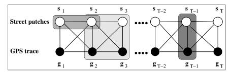
Figure 2: CRF for associating GPS measurements to street patches. The shaded areas indicate different types of cliques.
