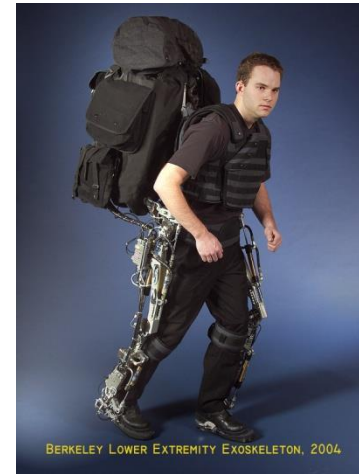
Berkeley Lower Extremity Exoskeleton 2004, can carry 150 lbs at 4 mph
