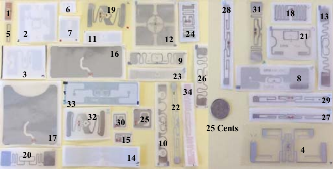
Fig. 1: The 34 EPC Gen2 passive tag types used for selection.
