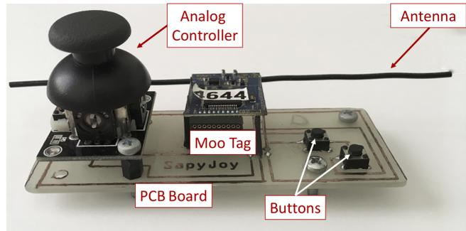
Fig. 1. SapyJoy videogame controller: A PCB board connects the analog controller and the buttons with the Moo tag.
